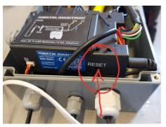
Fig. 6: Receiver "RESET" button
