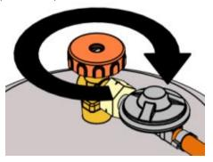
2. Turn the switch into the OFF position.
