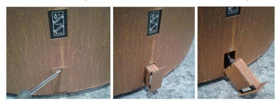
Fig. 8: Removing of the battery container
