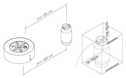
Fig. 4 – Gas cylinder distnace
