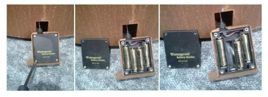
Fig. 9: Replacing the batteries in the container
