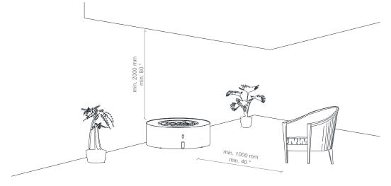
Fig. 1: Minimum distance to flammable materials
